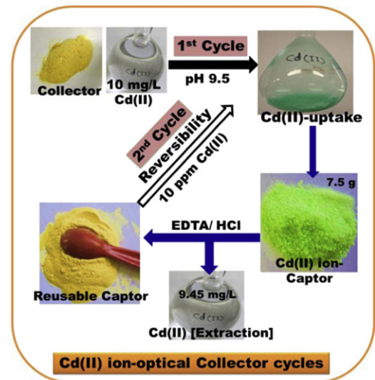
Scheme 2. Color profile of the TMPyP-modified-aluminosilicate mesocollector with the recovery/extraction system of [10 ppm] Cd(II) ions after several reuse/cycles (No.)
